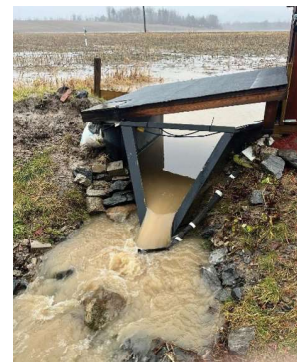
Above at left: Tile drainage outlet. At right: Surface drainage through monitoring equipment at UD.
